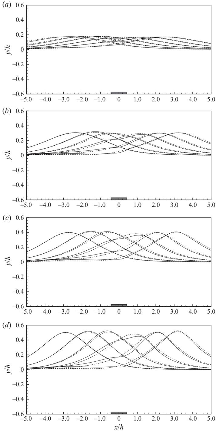
FIGURE 9. Free-surface profile at  $t\sqrt{g/h} = -2, -1, 0, 1, 2, 3$ , as computed by the present model (—) and by the potential-flow model (- - -). (a)  $H/h = 0.17$ , (b)  $H/h = 0.3$ , (c)  $H/h = 0.4$  and (d)  $H/h = 0.5$ .
