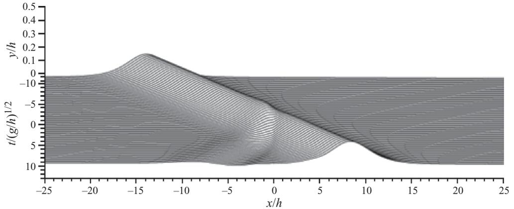
FIGURE 2. Free-surface profiles at various times for  $H/h = 0.17$ .
