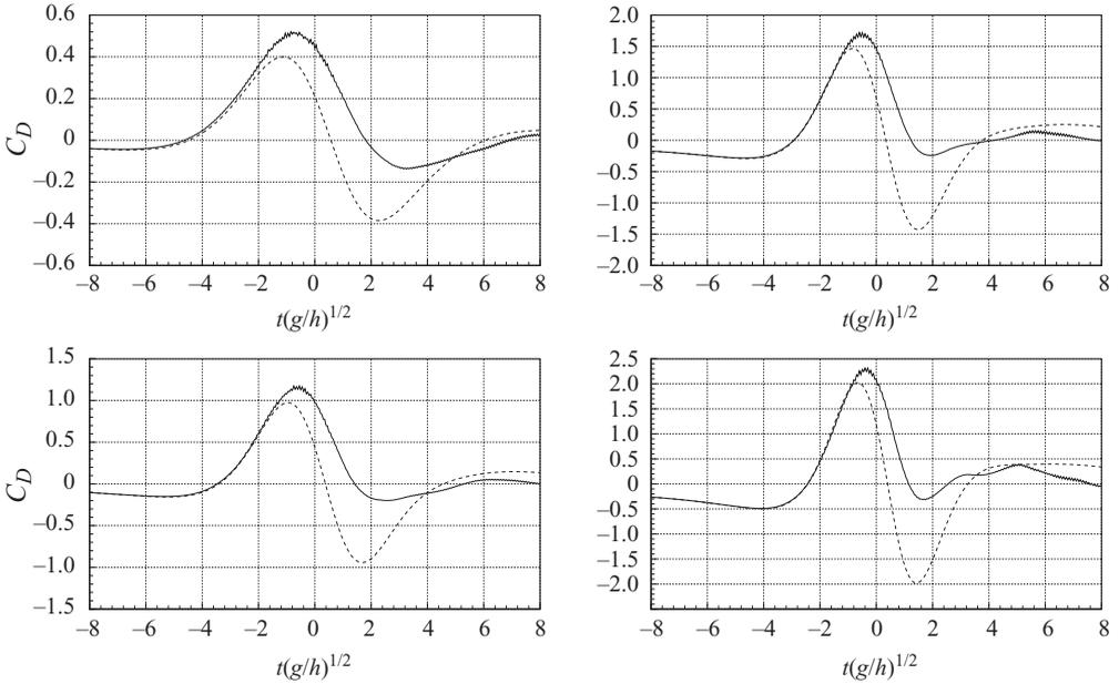
FIGURE 13. Comparison of the drag coefficient computed by —, present model; - - -, potential-flow model.
