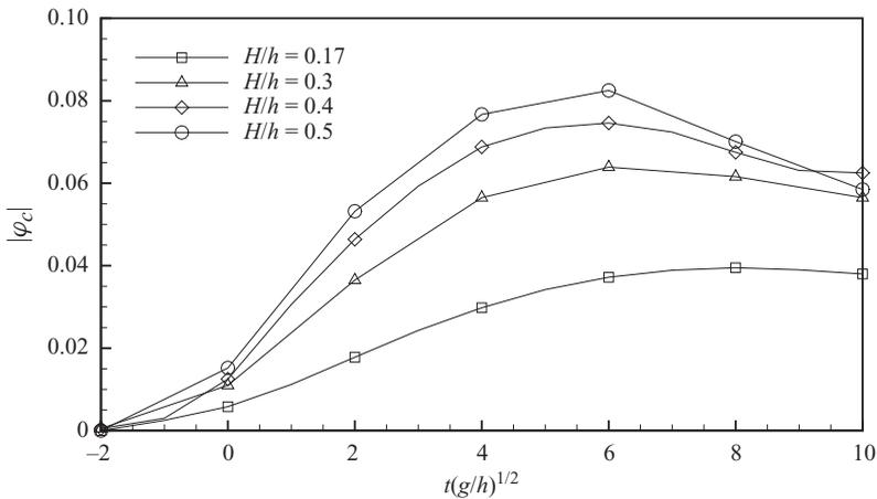
FIGURE 11. Time history of the maximum magnitude of the stream function in the core of the lee-side vortex for different wave heights.
