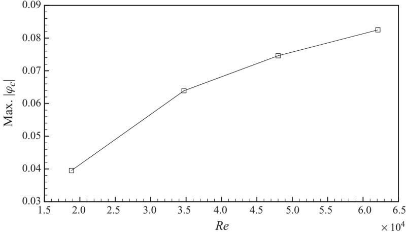
FIGURE 12. Maximum magnitude of the stream function in the core of the lee-side vortex as a function of the Reynolds number.
