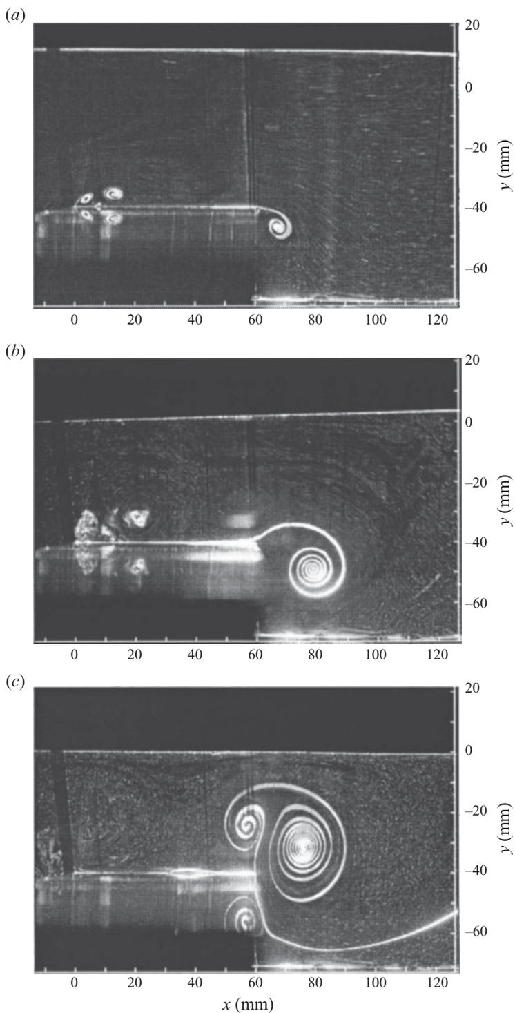
FIGURE 6. Global flow pattern obtained by LCHC using LIF at (a)  $t\sqrt{g/h} = -0.95$ , (b)  $t\sqrt{g/h} = 2.01$  and (c)  $t\sqrt{g/h} = 13.97$ .
