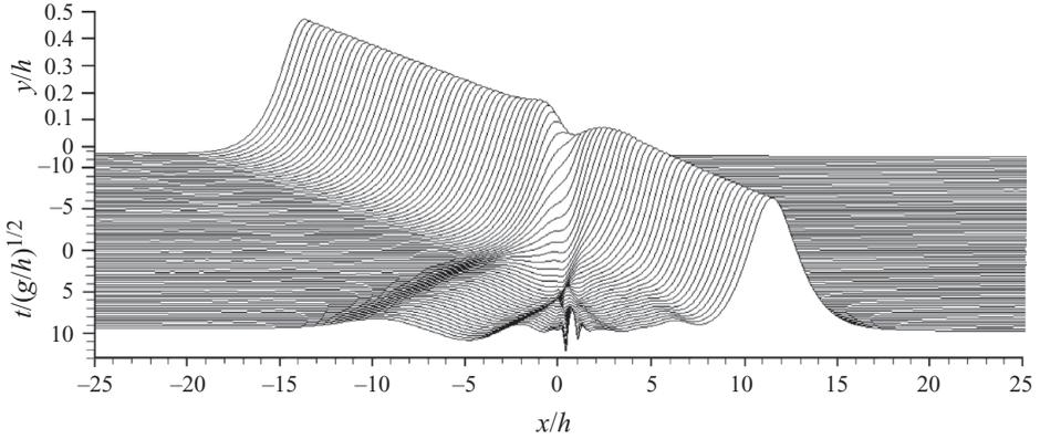
FIGURE 7. Free-surface profiles at various times for  $H/h = 0.5$ .
