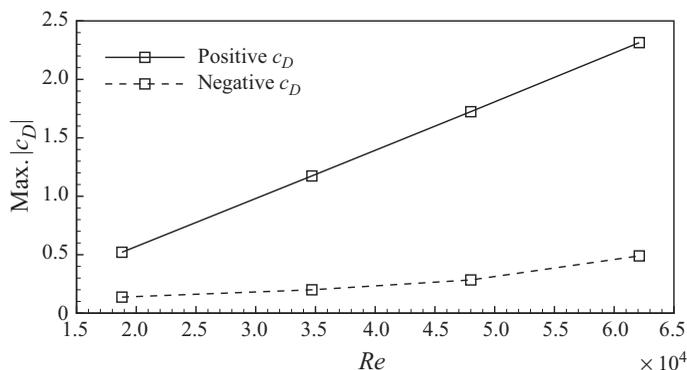
FIGURE 14. Maximum drag coefficient (positive and negative) versus the Reynolds number.
