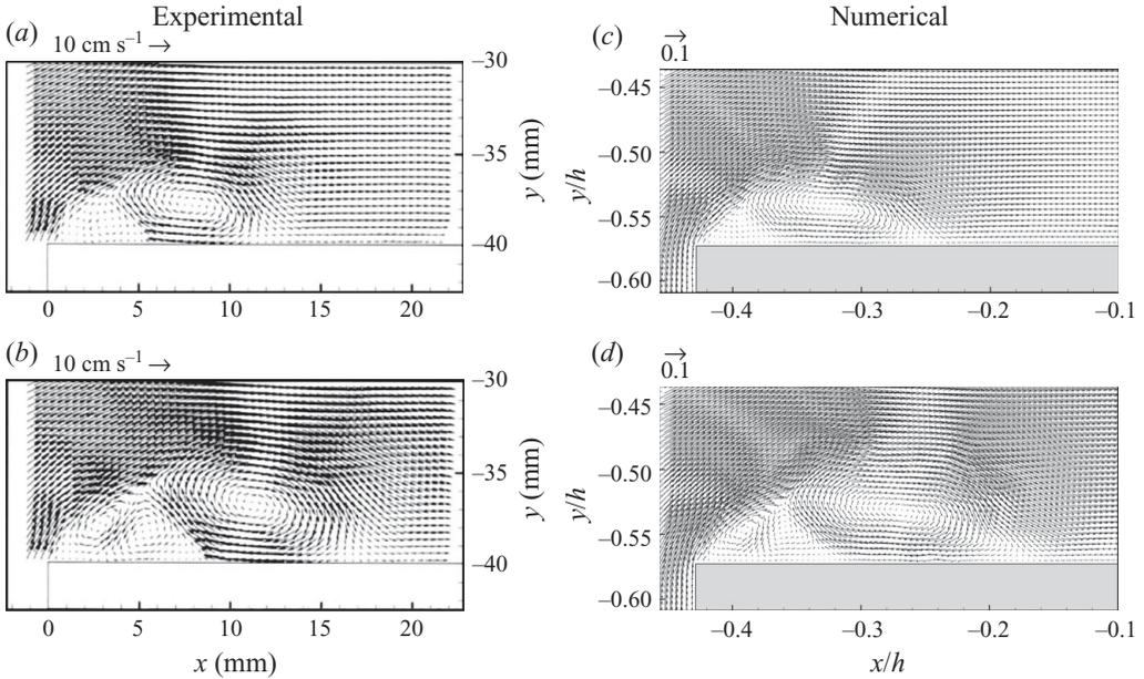
FIGURE 4. Comparison of the velocity fields at the leading edge of the obstacle between the experimental measurements by LCHC (*a, b*) and the numerical results for  $H/h=0.17$  (*c, d*). (*a*)  $t\sqrt{g/h}=-2.37$ , (*b*)  $t\sqrt{g/h}=-1.18$ , (*c*)  $t\sqrt{g/h}=-2.4$  and (*d*)  $t\sqrt{g/h}=-1.2$ .
