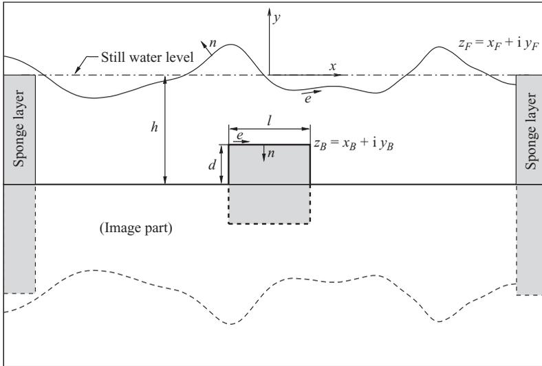
FIGURE 1. Definition sketch for water waves over a submerged obstacle.
