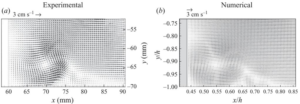
FIGURE 5. Comparison of the velocity fields near the sea-floor at the lee side of the obstacle between (*a*) the experimental measurements by LCHC (at  $t\sqrt{g/h}=12.43$ ) and (*b*) the numerical results for  $H/h=0.17$  (at  $t\sqrt{g/h}=12.5$ ).
